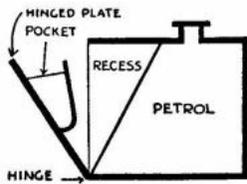
push Ormsby's steel rule right down to the bottom of the tank, and even feel round its edges, without discovering the trick.
